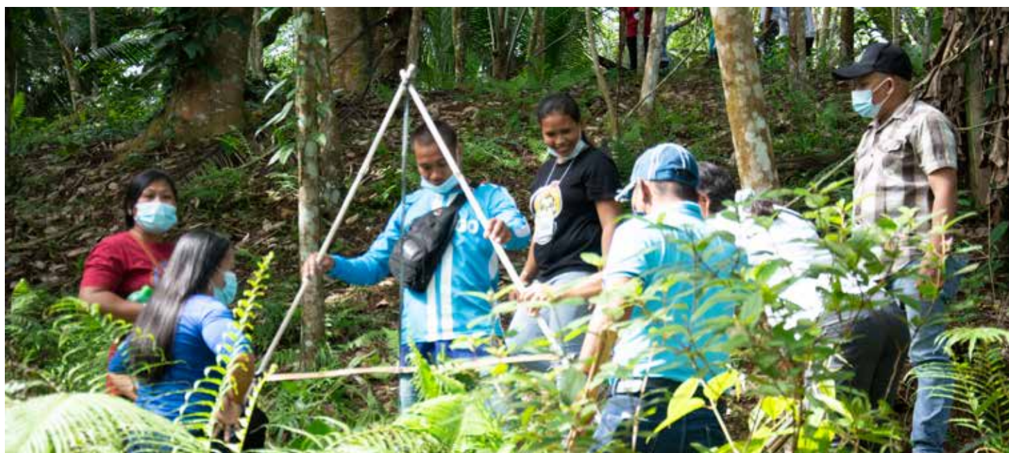
ATI XI Rice program Focal Person, Ernie L. Malazarte (extreme R) leads the participants during the demonstration of using A-frame level. It is an accurate tool to determine the contour of the slope areas.
