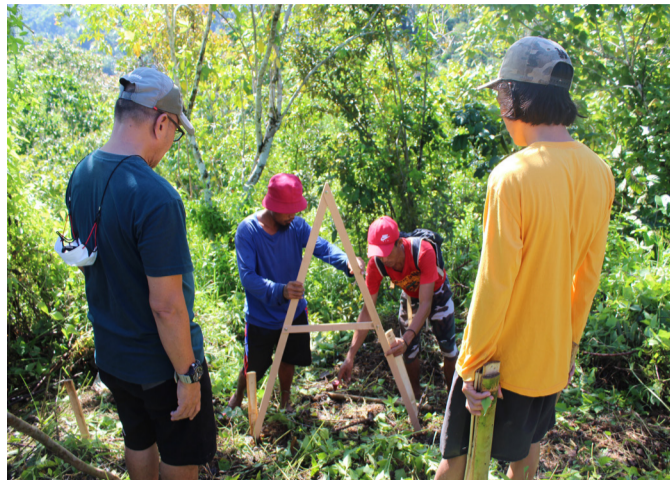
Participants perform the establishment of contour lines using A-frame during their practicum.
