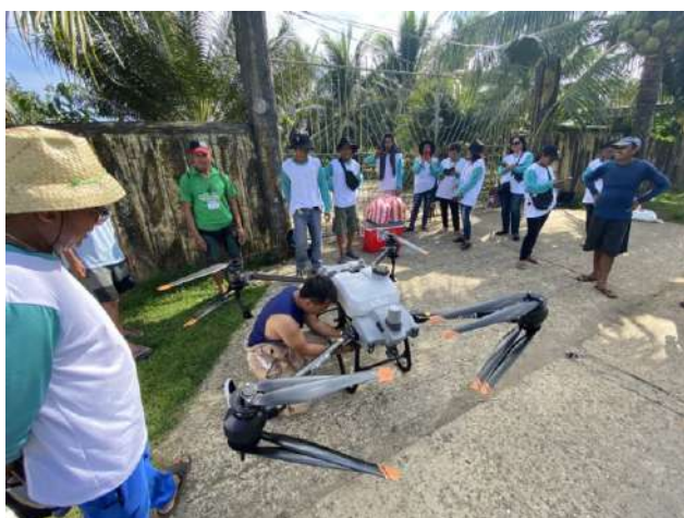
Drone service providers from New Hope showed participants how to setup the drone for fertilizer application during their demo in Lavesarez, Northern Samar.
